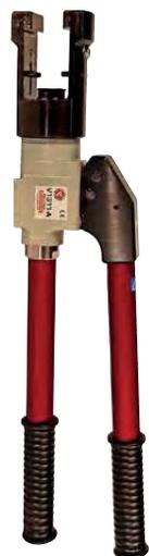
Tested and certified hydraulic hand-held tool for crimping Cu-terminals, type KR/KRT 10 mm<sup>2</sup>, KS/KST 10 mm<sup>2</sup>, KRF/KRD/KRT 16-400 mm<sup>2</sup>, KSF/KSD/KST 16-400 mm<sup>2</sup>, Al terminals 16-400 mm<sup>2</sup> (-240 solid), DIN 46235 10-300 mm<sup>2</sup>, C-sleeves up to 240 mm<sup>2</sup> total area (C95-120).
