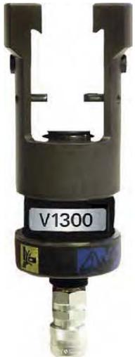
Tested and certified crimp head for crimping Cu-terminals, type KR/KRT 10 mm<sup>2</sup>, KS/KST 10 mm<sup>2</sup>, KRF/KRD/KRT 16-400 mm<sup>2</sup>, KSF/KSD/KST 16-400 mm<sup>2</sup>, Al-terminals 16-400 mm<sup>2</sup> (-240 solid), DIN 46235 10-300 mm<sup>2</sup>, C sleeves up to 240 mm<sup>2</sup> total area (C95-120). Used in combination with foot pump P4000 or the electrically powered pump PS710 (battery powered version of PS710E is also available).
