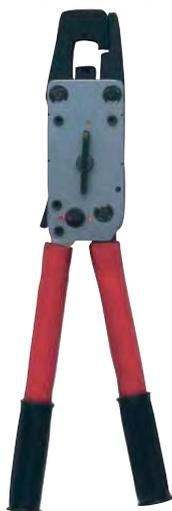
Mechanical hand-held tool for crimping Cu-terminals, type KR/KS 10 mm<sup>2</sup>, KRF/KSF 16-95 mm<sup>2</sup>, KR/KSD 16-120 mm<sup>2</sup>, KRT/KST 10-120 mm<sup>2</sup>, Al-terminals 16-25 mm<sup>2</sup> (-35 solid), and C-sleeves 6/6-50/50 mm<sup>2</sup>, DIN 46235 10-95 mm<sup>2</sup>.
