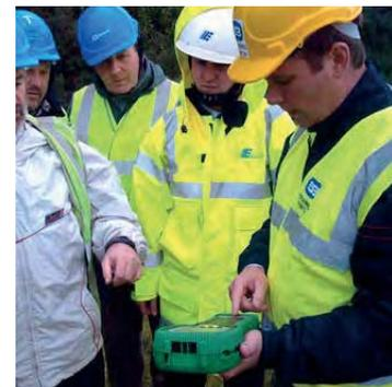
Measuring earthing resistance of the earth connection
