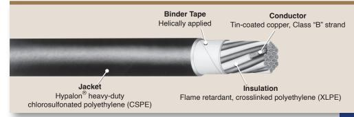
90°C\*, 600 Volt Class 1E Nuclear NEC Type TC UL Listed Spec. RSS-3-021
